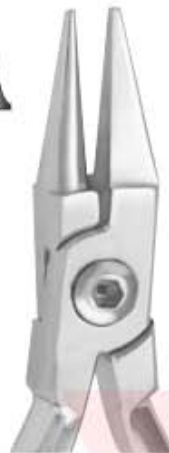
ID-20-0067 Bird beak plier for light wire bending round, square and rectangular up to .016"/0.41mm.
