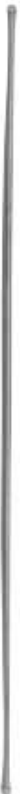
LG8-023-250 25.0 cm, 10" LG8-024-300 30.0 cm, 12" Double ended probes, tin, malleable, diam, of tips 3.5 mm with hole
